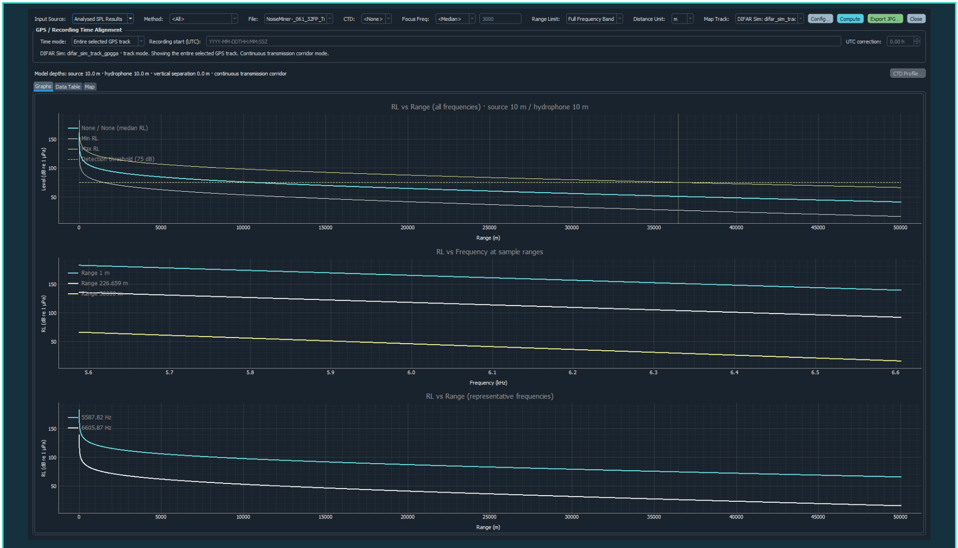
Figure 6. Computed NoiseMiner propagation results near 5.59 and 6.61 kHz, including receive-level curves, detection threshold, depth assumptions, and GPS-track alignment.
